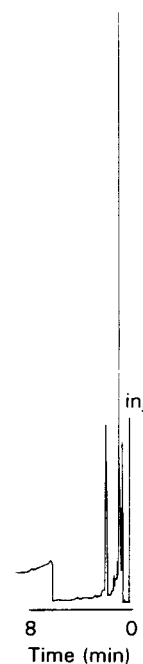
FIG. 2. Chromatogram showing the assay of Isosensitest broth. Column: 80 mm long, 4.6 mm i.d. packed with 5 \mu\text{m} ODS-Hypersil. Mobile phase: 5% acetonitrile, 10 mM disodium hydrogen orthophosphate, 20 mM TBA. Sensitivity: 1.28 changing to 0.04. Detection: 280 nm. Flow rate: 1.5 \text{mL min}^{-1} .
