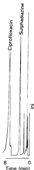
FIG. 1. Chromatogram showing the separation of sulphadiazine and ciprofloxacin in Isosensitest broth. Column: 80 mm long, 4.6 mm i.d. packed with 5 \mu\text{m} ODS-Hypersil. Mobile phase: 5% acetonitrile, 10 mM disodium hydrogen orthophosphate, 20 mM TBA. Sensitivity: 1.28 for sulphadiazine, 0.04 for ciprofloxacin. Detection: 280 nm. Flow rate: 1.5 \text{mL min}^{-1} .
